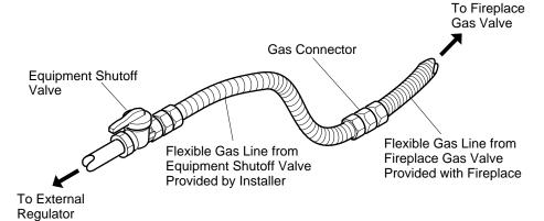
Figure 22 - Attaching Flexible Gas Lines Together
